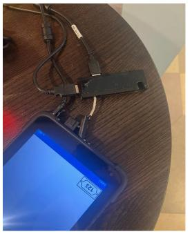
This 4-way USB hub should be plugged into the tablet, with two USB's connected to it. One is for the Epson printer, and the other is for the scanner. It is essential that these are ALWAYS connected to ensure proper functionality.
